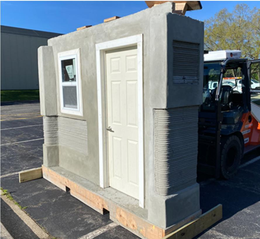
3D Printed Test Wall. Photo credit: Home Innovation Research Labs (2022).
