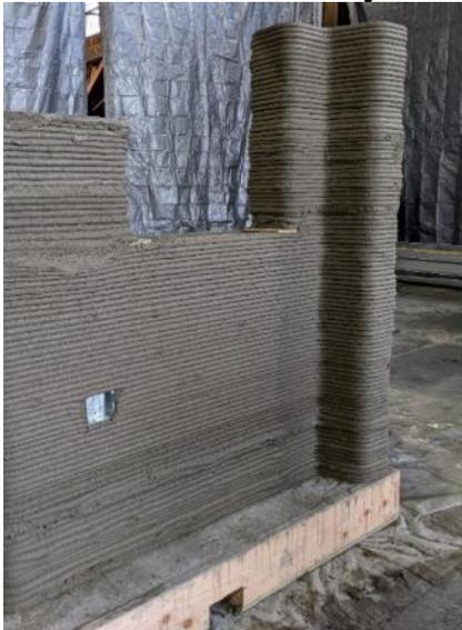
3D Printed Test Wall with Electrical Receptacle.
