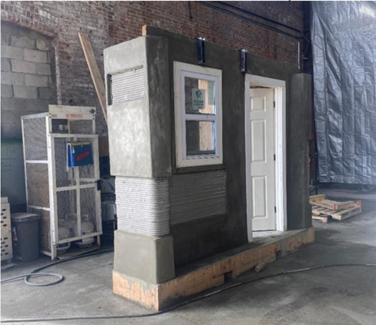
Various Surface Finishes on Test Wall.
