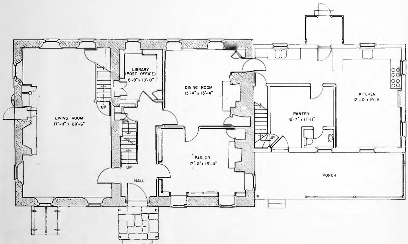
*Lundale Farm, Pennsylvania (ca. 1796). The walls of the older sections of this stone farmhouse are about eighteen inches thick with large chimneys set in them. Notice how much thinner the walls are in the 1950 addition and how small the new chimney is. The living room has two other energy saving features, splayed window reveals and a pass-through for firewood next to the chimney.*
