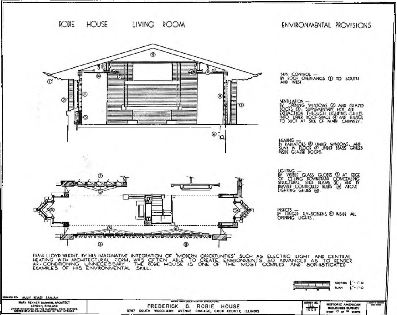
*Frederick C. Robie House, Illinois (1908-10). The overhangs are so precisely sized that the midday summer sun just touches the window sills on the south side. The windows and vents are located so that cool air can be drawn up through the house from the basement and exhausted at the ceiling or attic level.*
