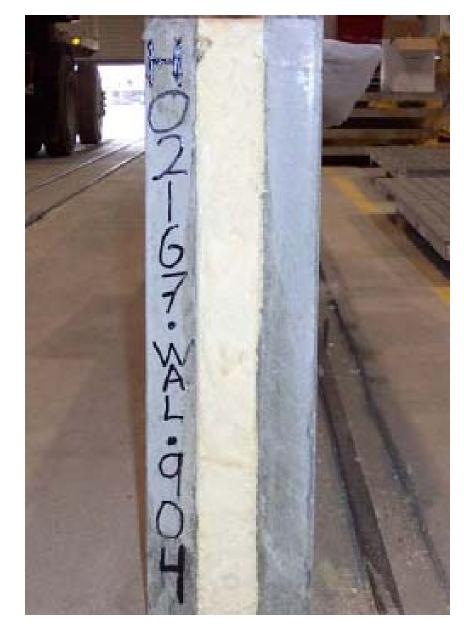
Insulation core between two concrete surfaces
