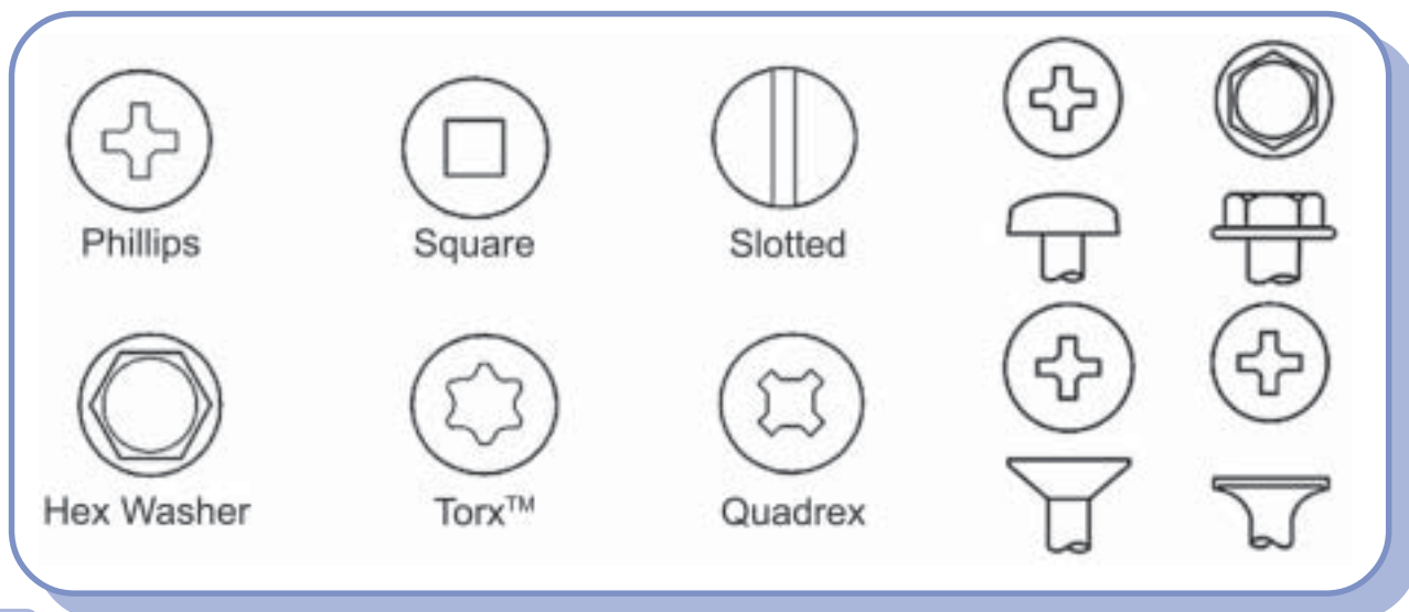
Figure 4.7– Screw Drive Types
