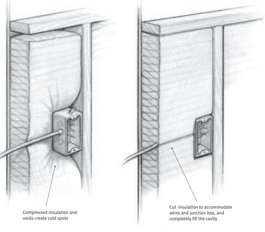
Compressing the insulation with wires and other material placed in the exterior walls will create cold spots on the inside wall covering (left). Cut insulation to fit around junction boxes and to completely fill the cavity (right).
