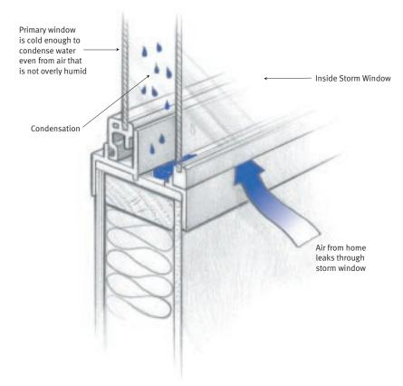
Pressure imbalance in a house will push warm air through leaks in the interior window allowing moisture to condense between the two panes of glass. A durable seal should be applied to the storm window to minimize leaks.
