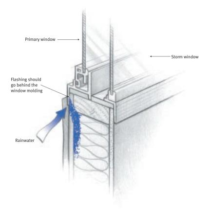
When windows aren't installed properly, rainwater can be driven behind the rain screen.
