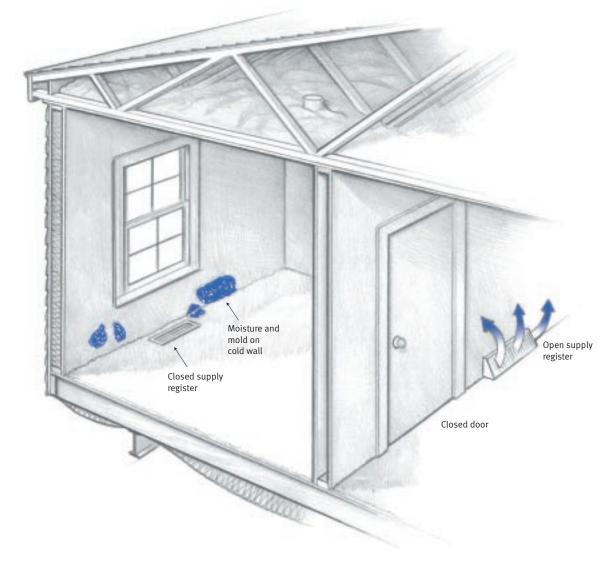
When the supply grilles are closed, warm air cannot enter a closed-off room. The inside air will become cold enough to significantly raise the relative humidity level in the room, supporting mold growth.
