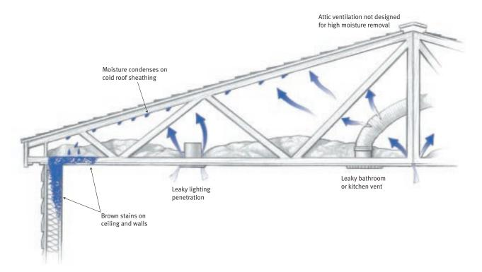
Warm, moist air that leaks from the home into the roof cavity will promote condensation on the underside of cold roof sheathing. Water runs down and is absorbed by the ceiling and wall sheathing, creating stains.
