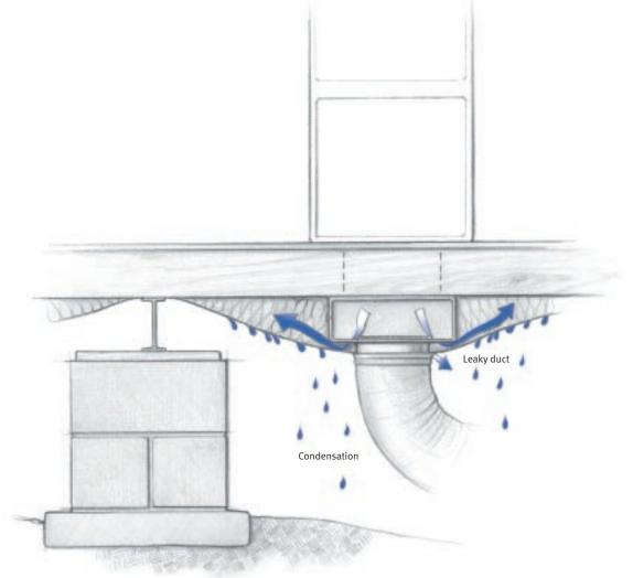
Duct leaks can cause water to "rain" into the crawlspace. Cold air that leaks from the underfloor duct system cools the belly material, supporting the condensation.
