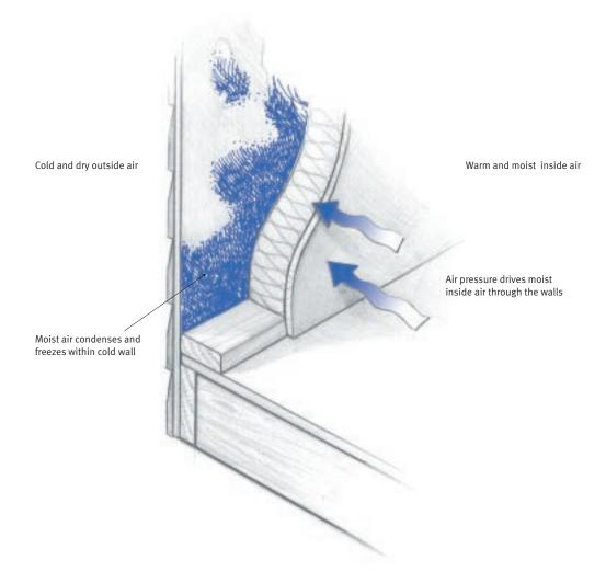
Static and vapor pressure drives moist inside air through the walls, where it condenses on the insulation and freezes. The frozen walls are cold to the touch, and the home will not feel warm.
