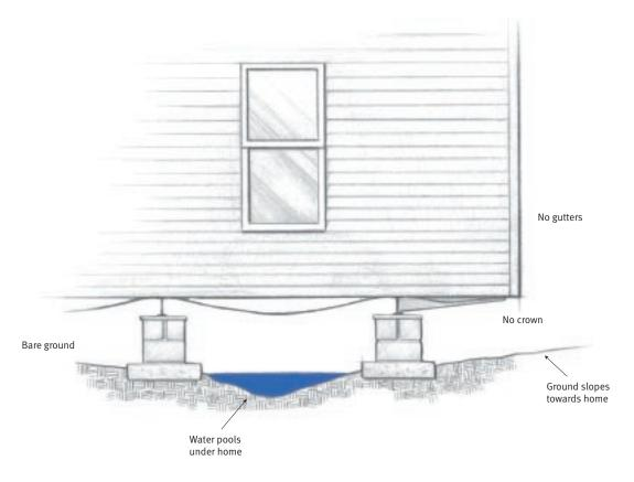
A properly graded site has a crown underneath the home and sloping ground that carries water away from the house, unlike the poor grading job shown above. Gutters and downspouts prevent splash back and direct water away from the foundation. Ground should be covered with a polyethelene sheet.
