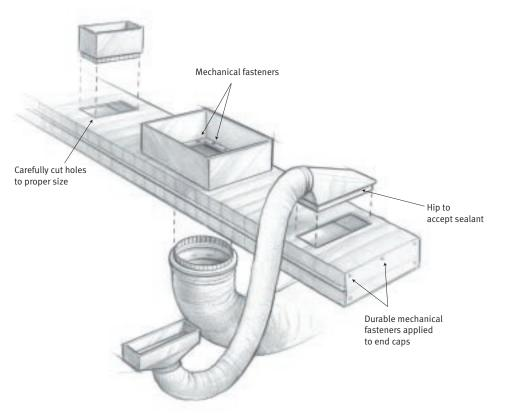
Leaky ducts increase the chance of moisture problems. To make airtight connections, cut accurate holes in the trunk, use boots and collars with a hip to accept sealant, and mechanically fasten connections.
