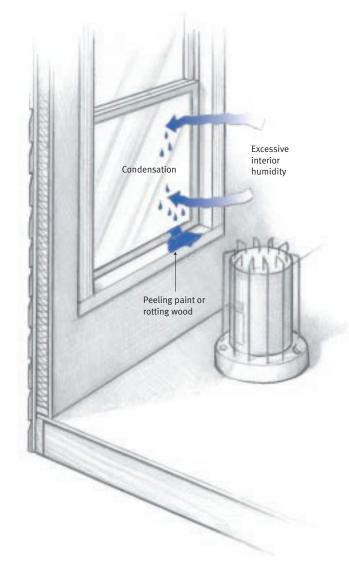
In winter, excessive interior humidity causes water to condense and run down inside the surface of the window glass and damage the sill. Unvented combustion space heaters that give off a good deal of moisture are sometimes the culprit.
