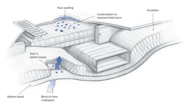
Warping of the floor sheathing can occur when a hole in the bottom board allows moist crawlspace air to condense on exposed metal ducts. Water is absorbed by the floor sheathing, which swells.
