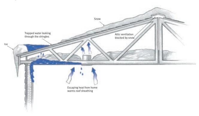
Ice dams occur when attic insulation is insufficient or warm home air enters the attic space. Melting snow or ice on the roof surface backs up and seeps through the shingles into the roof cavity, damaging materials and reducing insulation values.
