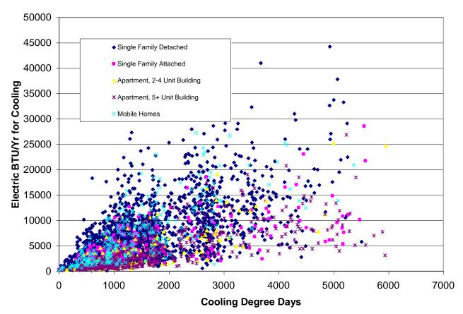
Again, the variation in electric use for air conditioning is considerable but displays an increasing relationship with cooling degree-days. For similar reasons as described in the heating section, the form of the regression equation was chosen to be:
