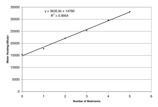
Figure 10 – Water Heating by Natural Gas Regression
