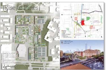
Site: The central design feature of Rise of Pines is the integration of Atlanta's existing Exhibition Hall into the site. The northern half of the Exhibition Hall is demolished at an existing expansion joint. The roof of the Exhibition Hall is reimagined as a one-acre park connected to the Civic Center Plaza by a terraced network of water, plants, stairs, and wheelchair-accessible ramps.
