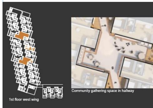
**Inclusivity:** The design incorporates a linked building approach for all four seasons. The hallways incorporate nodes, which create loose gathering areas, and there are larger, reflective spaces at the ends of the buildings' wings. Construction employs a modular approach and prefabricated units, which are interchangeable. The models and unit types have balconies in or out, with bedrooms facing in or out.
