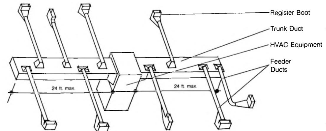
Figure 33. Extended Plenum Duct System
