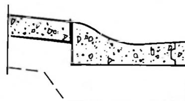
Figure 16b. Rolled curb blending with
