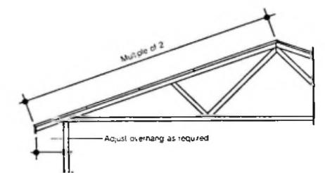
Figure 26. Engineered roof truss
