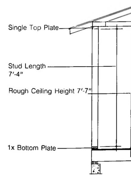
Figure 23. Wall construction for a 7'-6" finished ceiling height with studs vertically aligned over other framing members, permitting single top plate.
