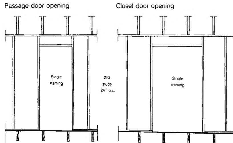
Figure 30. Single-framed openings in 2 x 3 non-load bearing partitions for passage doors and closets.
