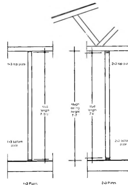
Figure 29. 2 x 3 partition construction with studs spaced 24" o.c. and alternate 1 x 3 plates.
