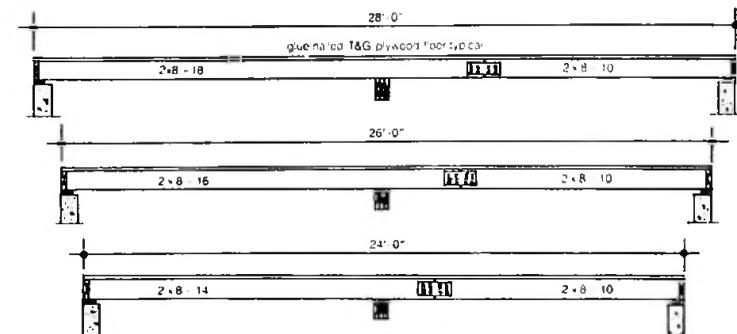
Figure 22. Off-center spliced joist designs span further than simple joists of the same dimension.
