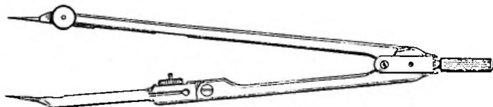
FIG. 31. COMPASS WITH DIVIDER POINTS
