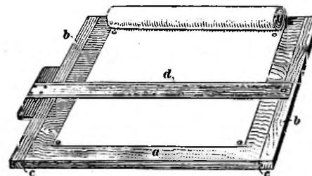
FIG. 3. SMALL DRAWING BOARD
