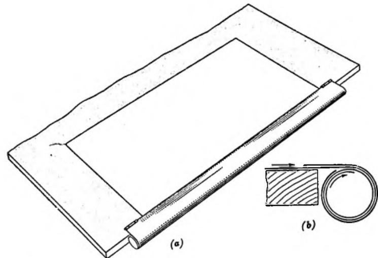
FIG. 39. GUARD FOR DRAWINGS
