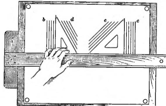
FIG. 9. USE OF TRIANGLES FOR VERTICAL OR SLOPING LINES
