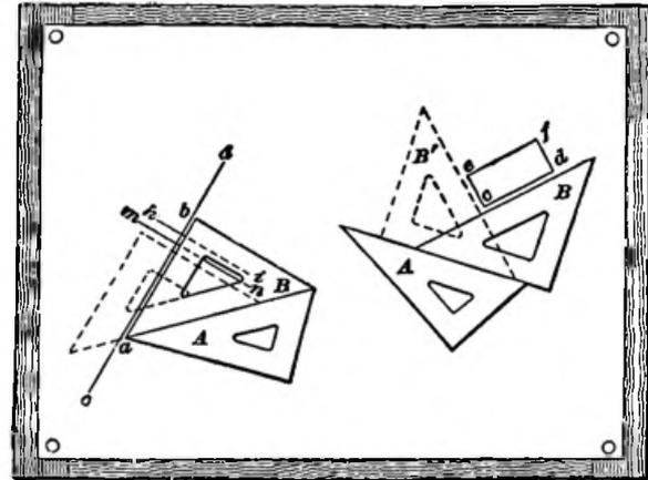
FIG. 11. USE OF TRIANGLES FOR LINES PERPENDICULAR TO GIVEN LINES
