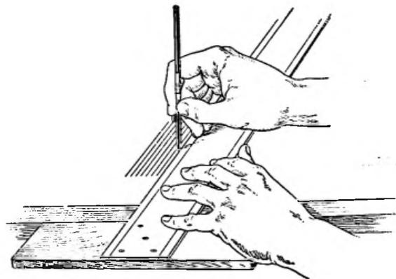
FIG. 33. RULING PEN IN PROPER, OR VERTICAL, POSITION
