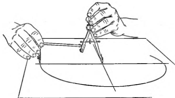
FIG. 27. USE OF LENGTHENING BAR
