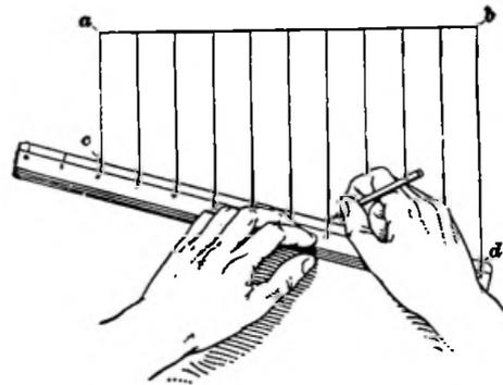
FIG. 17. SPACING BY MEANS OF SCALE
