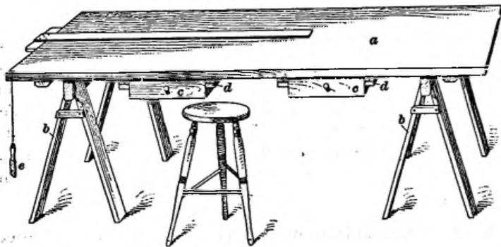
FIG. 1. ARCHITECT'S DRAWING BOARD
