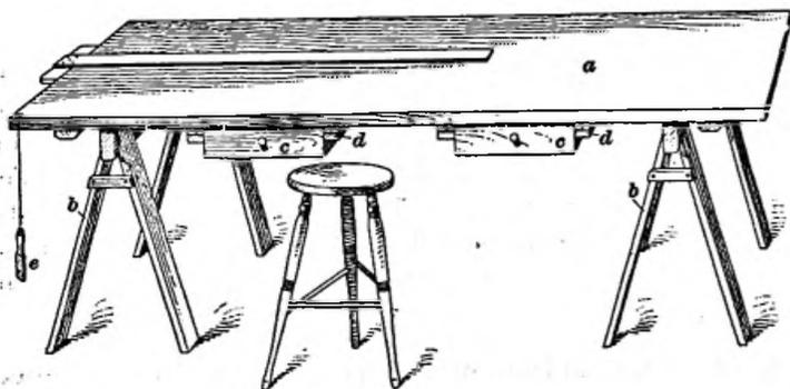
FIG. 1. ARCHITECT'S DRAWING BOARD
