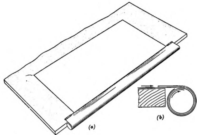
FIG. 39. GUARD FOR DRAWINGS
