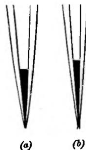
FIG. 34. PROPER AND IMPROPER ADJUSTMENT OF RULING PEN
