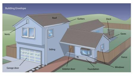
**Figure 1. Building Envelope** *Source: FEMA. Home Builder's Guide to Construction in Wildfire Zones.*
