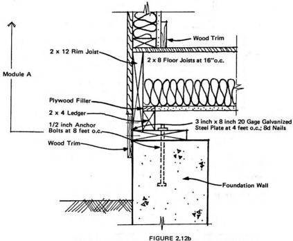
HERCULES- EXTERIOR MODULE TO FOUNDATION DETAIL
