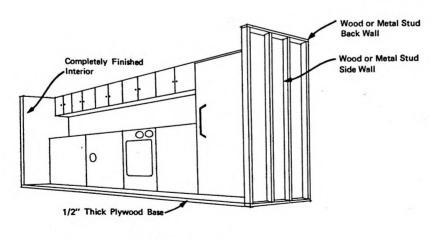
FIGURE 6.8 DESCON/CONCORDIA-KITCHEN MODULE
