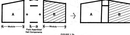
FIGURE 1.3b SITE ASSEMBLED HALLWAY BETWEEN MODULES
