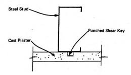
FIGURE 3.15b SECTION A-A-THROUGH PUNCHED SHEAR KEY
