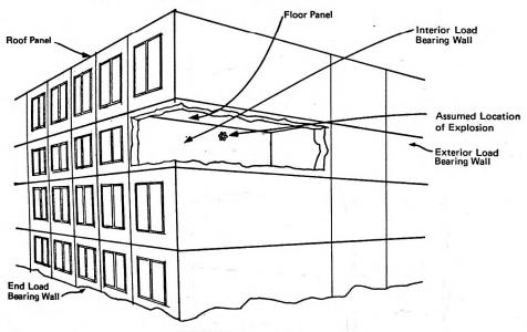
FIGURE 2.17f BUILDING SYSTEMS INTERNATIONAL-CORNER PANELS REMOVED BY ABNORMAL LOADING
