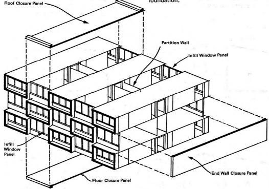
FIGURE 1.2b COMPLETION OF STRUCTURAL ASSEMBLY
