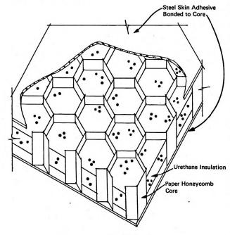
FIGURE 3.13 REPUBLIC STEEL-SANDWICH PANEL CROSS SECTION
