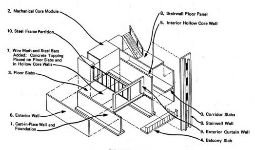
FIGURE 2.16 SCHEMATIC OF ERECTION PROCEDURE
