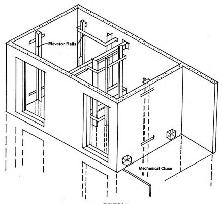
FIGURE 8.1 TYPICAL PRECAST DOUBLE ELEVATOR SECTION
