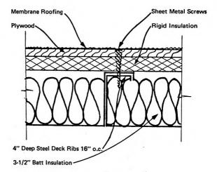
FIGURE 3.8 PANTEK ROOF DECK CROSS SECTION
