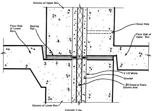
FIGURE 2.15g SHELLEY - COLUMN TO COLUMN JOINT
