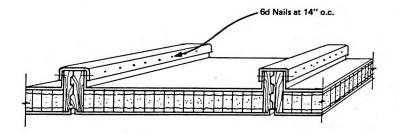
FIGURE 3.9b ASSEMBLED ROOF PANEL
