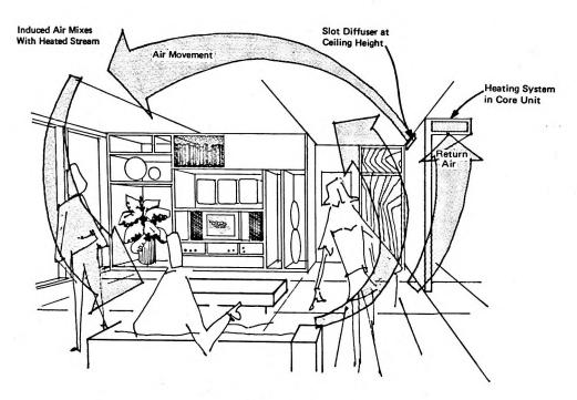
FIGURE 5.5 AIR MOVEMENT DUE TO THE "COANDA EFFECT"
