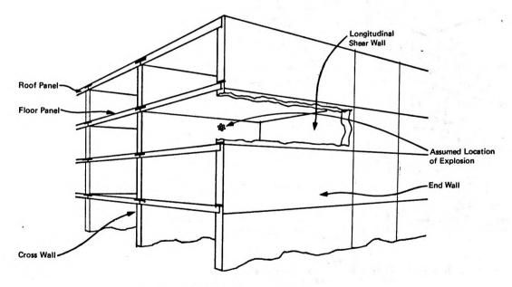
FIGURE 2.17e CAMCI-CORNER PANEL REMOVED BY ABNORMAL LOADING
