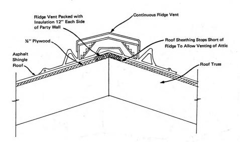
FIGURE 3.4 CONTINUOUS RIDGE VENT PACKED WITH INSULATION
