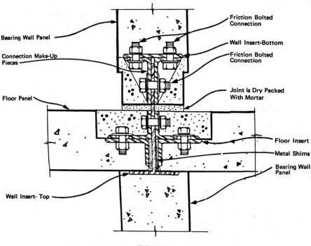
FIGURE 2.156 DESCON/CONCORDIA- INTERIOR WALL TO FLOOR CONNECTION
