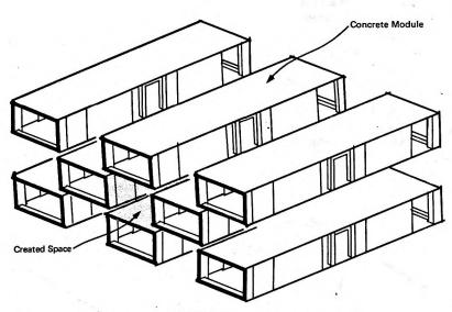
FIGURE 1,2a CHECKERBOARD ARRANGEMENT OF MODULES
