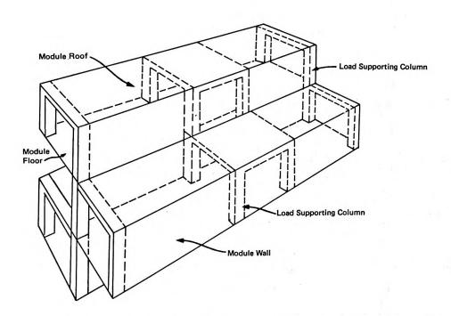
FIGURE 2.17a SHELLEY-VERTICAL ALIGNMENT OF MODULE COLUMNS
