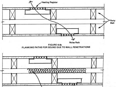
Insulation to Block Sound Transmission
