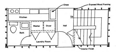
FIGURE 6.3b FLOOR PLAN-MECHANICAL CORE MODULE WITH STAIRS
