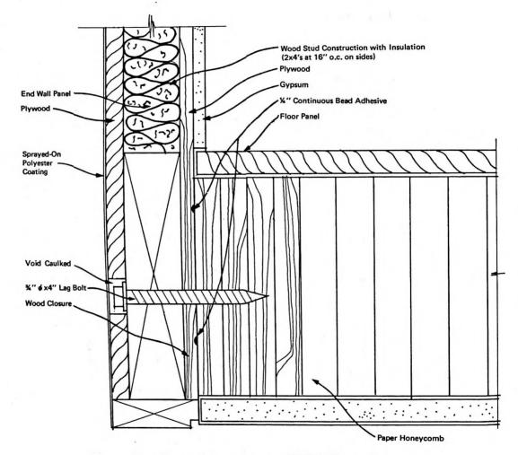
FIGURE 2.10f TRW- TYPICAL END WALL PANEL TO FLOOR DETAIL
