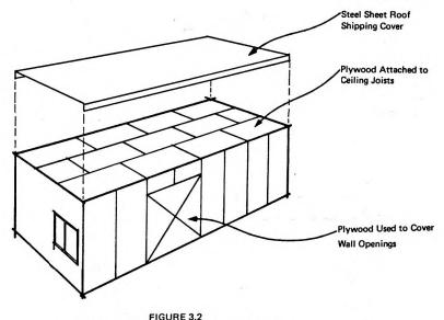
SHEET METAL SHIPPING ROOF ON MODULE
