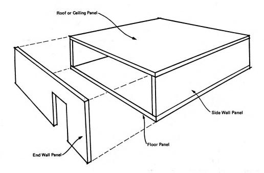
FIGURE 2.10 d TRW- FIBER-SHELL MODULE CONSTRUCTION
