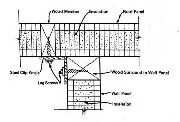
FIGURE 2.10a REPUBLIC STEEL-WALL/ROOF CONNECTION
