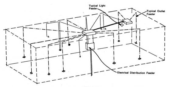
FIGURE 7.4 HARNESS INSTALLED IN MODULE
