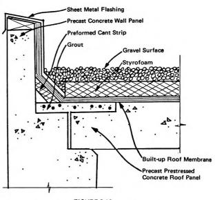
FIGURE 3.10 INSULATED ROOF MEMBRANE ASSEMBLY
