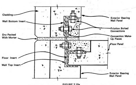
FIGURE 2.15a DESCON/CONCORDIA- EXTERIOR WALL TO FLOOR CONNECTION
