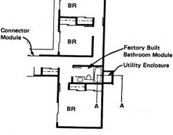
FIGURE 6.5a FACTORY BUILT BATHROOM MODULE
