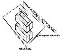
FIGURE 6.3a MECHANICAL CORE MODULES PLACED TWO HIGH
