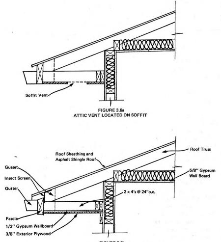
FIGURE 3.6b ATTIC VENT RELOCATED FROM SOFFIT TO FASCIA
