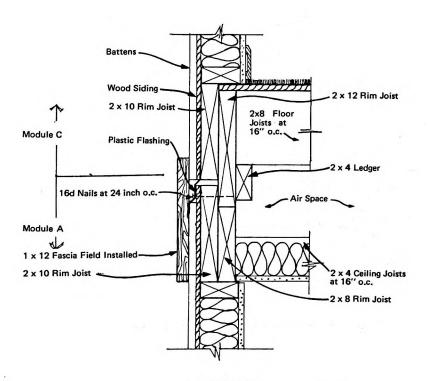
FIGURE 2.12h LEVITT- EXTERIOR MODULE TO MODULE DETAIL
