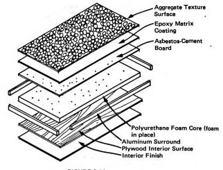
FIGURE 3.14 PANTEK-SANDWICH PANEL CONSTRUCTION OF EXTERIOR WALLS
