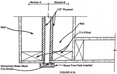
LEVITT-SHEET METAL FIRE SHIELDS AT INTER-MODULE JOINT
