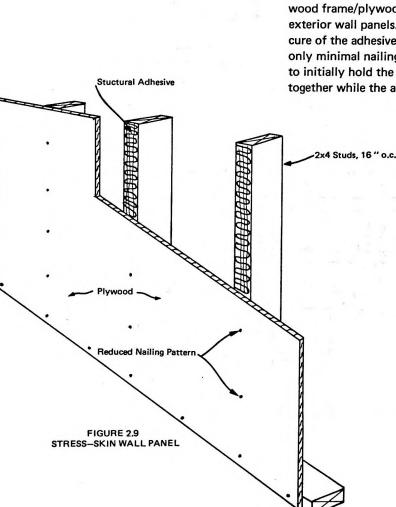
housing has led to the use of an adhesive that has the structural strength of a resorcinol (a timeproven wood adhesive) and the set-up speed of a contact adhesive. This product, used by Pemtom, provides stiffness for the structural elements by creating wood frame/plywood stress skin exterior wall panels. The rapid cure of the adhesive means that only minimal nailing is needed to initially hold the components together while the adhesive sets.
