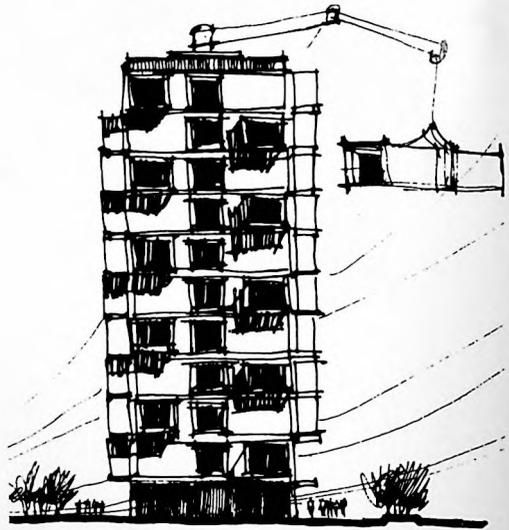
The initial mechanism selected by this producer for lifting the modules was a simple cable arrangement which connected to two points on each side of the unit and then to a single heavy tubular spreader bar. The crane cable pick-up points were located at the ends of the spreader bar. However, it was found that this "double triangle" cable method, although light in weight and relatively inexpensive, did not provide the desired stability needed during placement and movement of the units.
