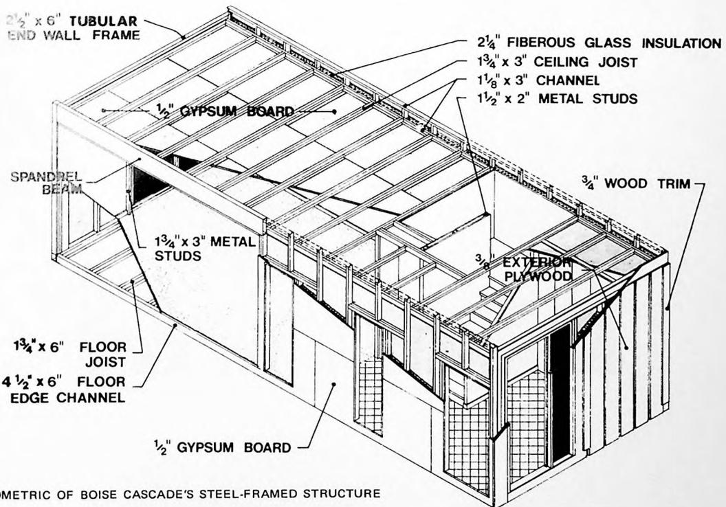
ISOMETRIC OF BOISE CASCADE'S STEEL-FRAMED STRUCTURE
