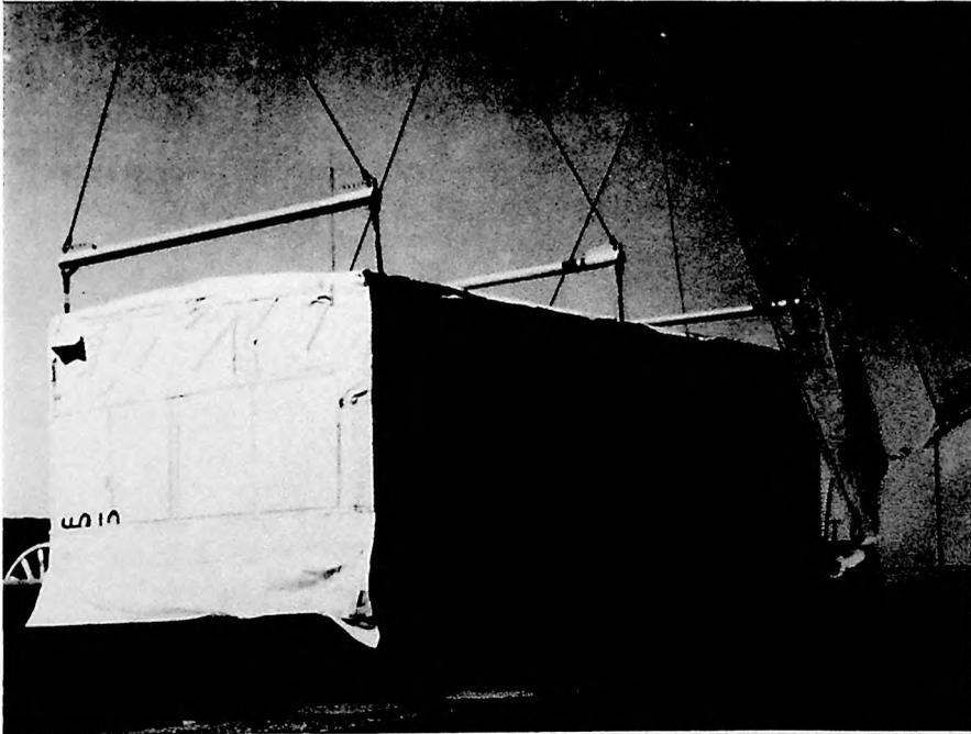
LIFTING FRAME WITH NYLON STRAPS
