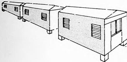
LOUVERS INSTALLED TO REDUCE INTERIOR MOISTURE ENTRAPMENT
