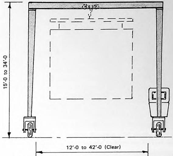
TYPICAL DIMENSIONS OF "TRAVEL LIFTS" AVAILABLE FOR YARD STORAGE AND PLANT HANDLING OF MODULAR HOUSING UNITS
