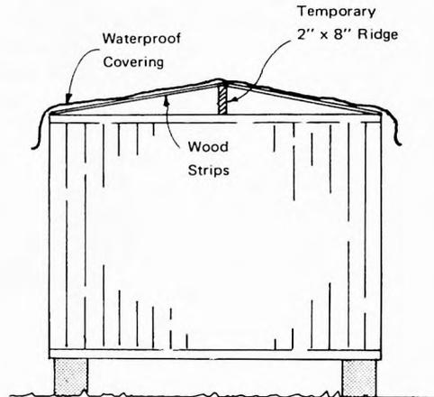
MSC MODULE SHOWING TEMPORARY ROOF COVERING STRUCTURE
