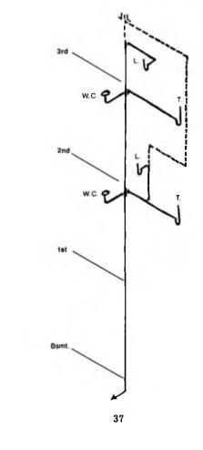
Typical Fully Vented Back-to-Back Bathroom Stack with Alternate Solution
