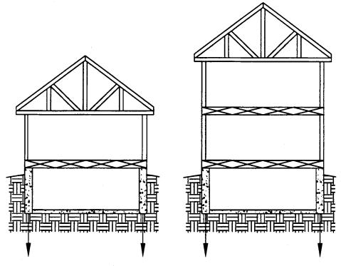
Figure 8. Typical House Sections: Trussed Floors and Roof.
