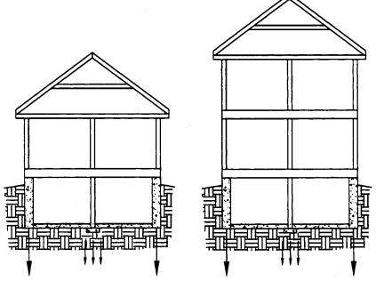
Figure 6. Typical House Sections: Stick-Built Floors & Roof
