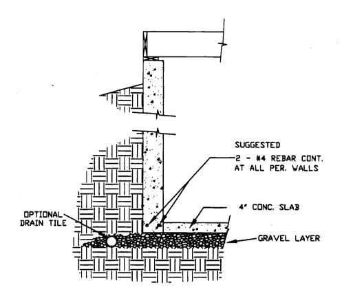
Figure 16. Two- and One-and-One-Half-Story Stemwall Recommendations
