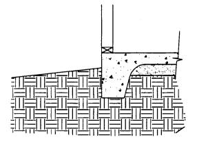
Figure 5. Slab-on-Grade Construction.
