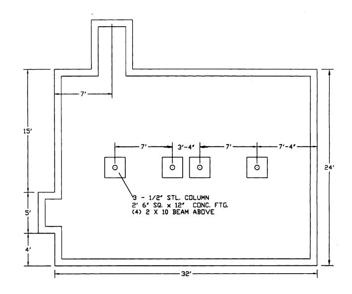
Figure 15. Massachusetts Foundation Plan
