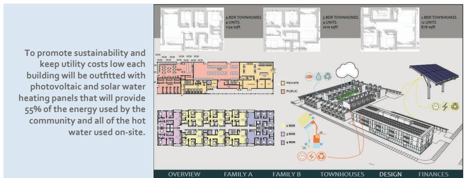
To promote sustainability and keep utility costs low each building will be outfitted with photovoltaic and solar water heating panels that will provide 55% of the energy used by the community and all of the hot water used on-site.
