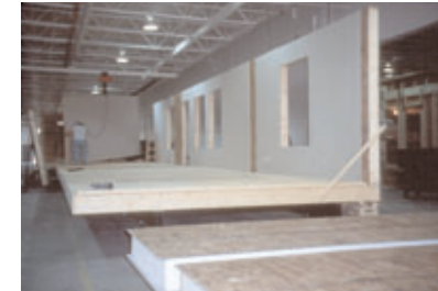
Structural insulated panels improve energy efficiency (courtesy, SWA).
