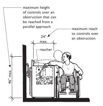
Use of Top-Loading Machine Made Possible With Assistance of a Mechanical Reacher
