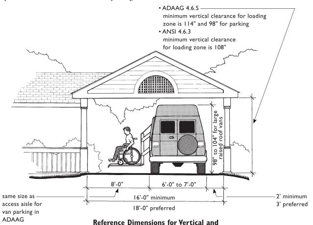
Horizontal Clearances for Raised Roof Van with Lift Extended
