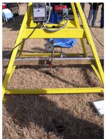
Figure 2.7. 90 degree in-line (axial) pull test set-up.
