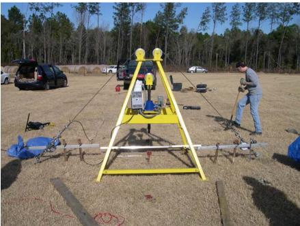
**Figure 2.8.** Angle pull test set-up (NOTE: Anchors are being tested as an in-line angle pull installation so the horizontal ruler used for deflection measurement is set-up to the inside of the anchors to avoid potential ground surface disturbance caused by the anchor)
