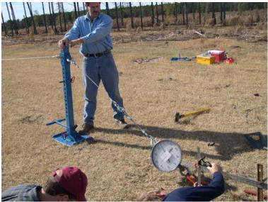
Figure 5.1. Lever Arm Test Rig (Tie Down Engineering, Inc.)
