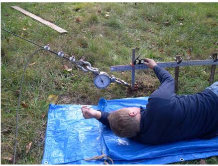
**Figure 2.9.** Deflection measurement technique for angle pull tests. (*NOTE:* Anchor being tested is a not in-line with the angle of pull so a stabilizer plate is used and the horizontal ruler for measuring anchor deflection is set-up to the outside of the anchor)
