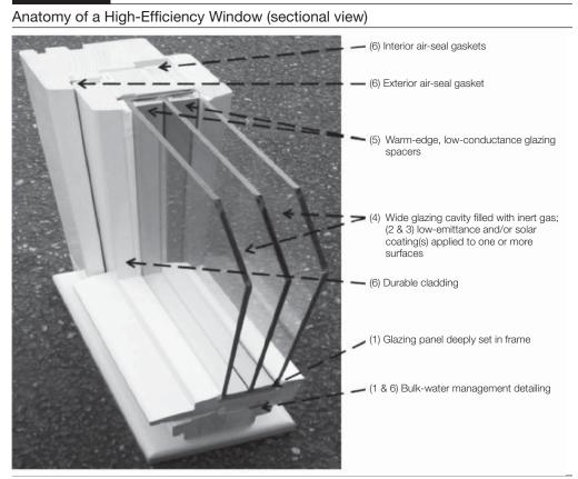
Note: Numbers indicate technological improvements as follows: (1) glazing unit structure; (2) low-emittance (also called lowemissivity, or low-E) coatings; (3) solar-control glazings and coatings; (4) low-conductance gas fills; (5) warm-edge spacers; and (6) thermally improved sash, frame, and weather stripping.
