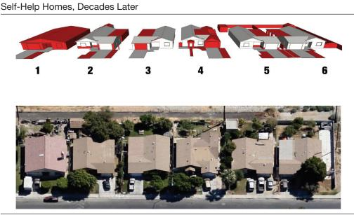
Six neighboring homes developed by a nonprofit housing developer in California in the late 1980s. The bottom image shows present-day aerial imagery. The top image shows a three-dimensional model analyzing the incremental changes; features in white and gray represent the original homes, and features in red represent post-occupancy modifications made by the owners. Sources: Top—Mukhija and Scott-Railton (2013); bottom—Google Maps
