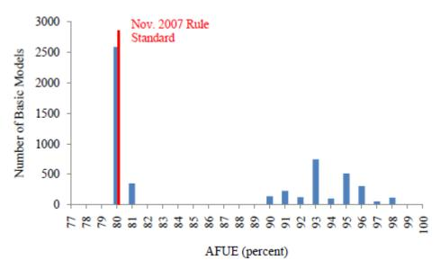
Figure 10. Distribution of Non-Weatherized Gas Furnace Models by AFUE
