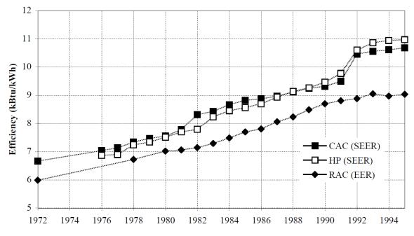
Figure 4. Shipment Weighted Efficiencies for Cooling Equipment 1972-1995
