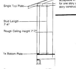
Figure 23. Wall construction for a 7'-6" finished ceiling height with studs vertically aligned over other framing members, permitting single top plate.
