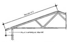
Figure 26. Engineered roof truss
