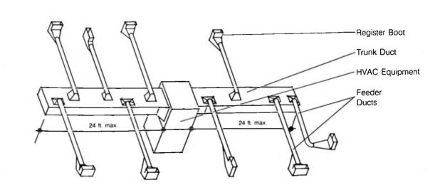
Figure 33. Extended Plenum Duct System
