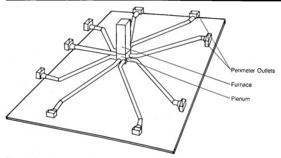
Figure 34. Typical Radial Duct System
