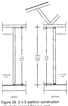
with studs spaced 24" o.c. and alternate 1 x 3 plates.
