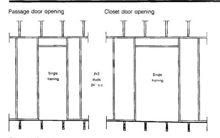
Figure 30. Single-framed openings in 2 x 3 non-load bearing partitions for passage doors and closets.
