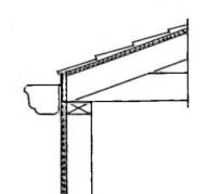
Figure 27a. Simple fascia board Figure 27b. Fascia eliminated Consider elimination of the rake overhang on a gable roof. The rake overhang is a costly detail, and serves no real function. A simple 1 x fascia may be used to trim the rake or trim may be entirely eliminated by fitting the siding to the underside of roof shingles.
