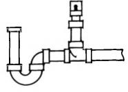
Figure 32. Typical Automatic Vent
