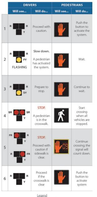
SY Steady yellowSRSteady redFY Flashing yellowFRFlashing red
