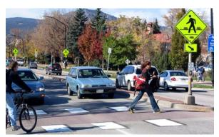
Flashing diodes in pavement\* and warning sign. Photo source: Dan Burden
