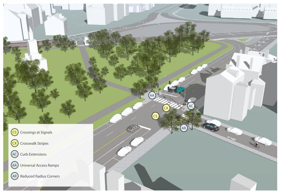
Raised Crosswalk / Speed Table (ст) (cs) Crossings at Signals Crossings at Stop/Yield Signs (CY) (CM) Mid-block Crossing Crosswalk Stripes (cx) AR (AA) Universal Access Ramps (AR) Reduced Radius Corners Pedestrian Only Crossing - Standard Signals (DP) Pedestrian Advance Walk (TG)
