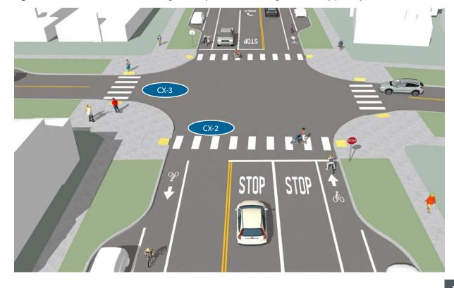
Figure B-24: Pedestrian bulb-outs with high visibility crosswalk markings at a two-way partially controlled intersection.
