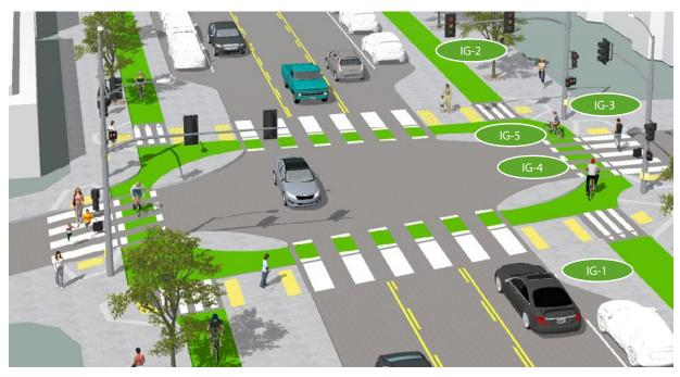
Figure B-13: Partial separated intersection combined with a two-way cycle track and a bike/pedestrian crosswalk. Please note FHWA Separated Bike Lane Planning and Design Guide, as well as emerging best practices for accessibility.
