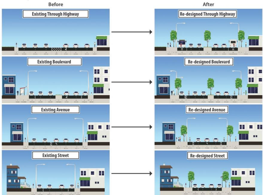
\*For Federal guidance on road diets, see FHWA's Road Diet Informational Guide: http://safety.fhwa.dot.gov/road\_diets/info\_guide/ Note: While actual widths permitted or required may vary from city to city, travel lanes of 11' or less are recommended for traffic calming, safety and pedestrian/bicyclist stress reduction.
