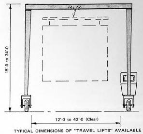
FOR YARD STORAGE AND PLANT HANDLING OF MODULAR HOUSING UNITS
