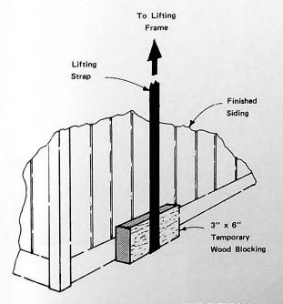
TEMPORARY BLOCKING TO PROTECT EXTERIOR FINISH DURING ERECTION
