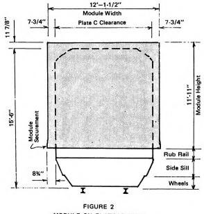
MODULE ON FLATCAR WITH PLATE C DIAGRAM
