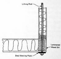
EMBEDDED LIFTING ROD DETAIL
