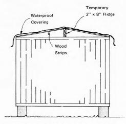
MSC MODULE SHOWING TEMPORARY ROOF COVERING STRUCTURE
