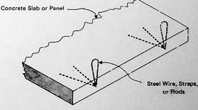
HANDLING & ERECTION LOOPS
