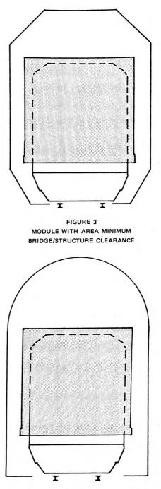
FIGURE 4 MODULE WITH AREA MINIMUM SINGLE TRACK TUNNEL CLEARANCE
