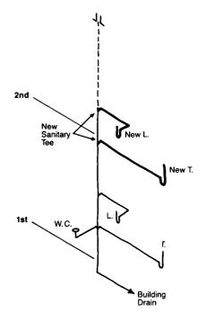
Addition of First Floor Powder Room of Single Dwelling Unit, with Basement Illustration of use of wet venting in solving a problem of the type discussed under 2.3. For possible use of single stack solutions, see 1.3(4) and discussion under 2.3.
