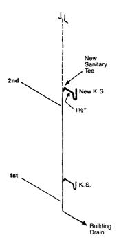
Most codes limit the pressure fluctuation within drainage systems to  $\pm\,1$  inch of water pressure under design load conditions. A more practical limitation, and the one used in this guideline, is to limit the trap seal reduction to 1 inch of water under normal conditions of loading. This concept permits the planning and carrying out of simple field tests on existing systems to determine their condition and provides a basis for approving modified systems in rehabilitated buildings.
