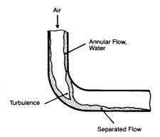
The disturbance at the base of the stack may be large, and significant positive pressures may be generated which, if not relieved, can cause blowback—the reversed passage of water through the trap. If the transition is smooth, much of the air is carried away through the horizontal drain.
