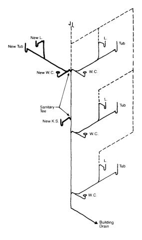
Addition of Second Floor Fixture to Existing Stack
