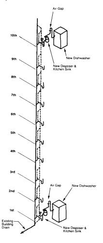
Engineered Single Stack System Sized According to Published Criteria
