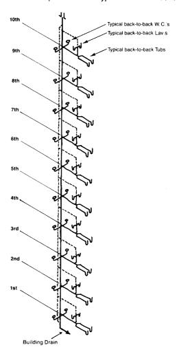
Typical Fully Vented Back-to-Back Bathroom Stack with Alternate Solution
